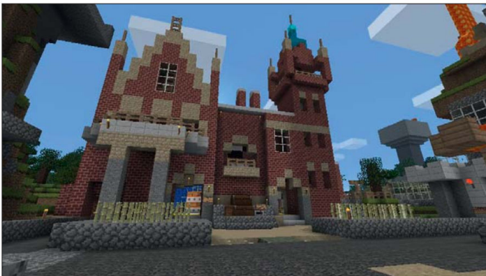
Figure 14.21: The game Minecraft models the entire world with 1\text{ m}^3 voxels, enabling efficient, real-time illumination, simulation, and rendering for fully dynamic Earth-scale worlds.
